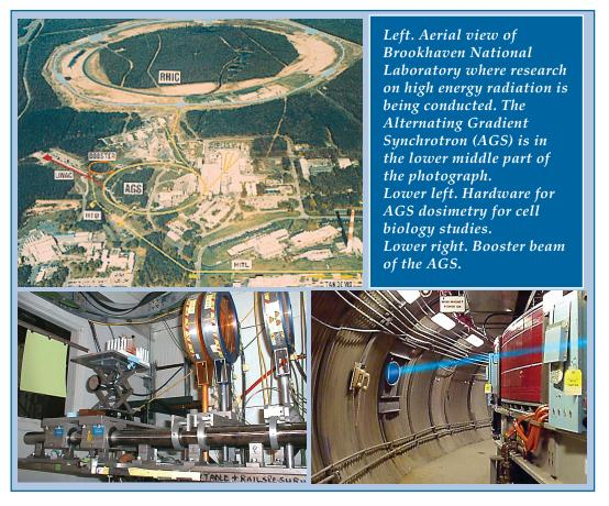
Energy facility possesses several particle accelerators that accelerate beams of atomic nuclei to successively higher energies. NASA-supported researchers have used one of these particle accelerators, the Alternating Gradient Synchrotron (AGS), for the past 8 years to collect data on the effects of exposure to high-energy radiation beams on cells, tissues, and experimental animals.
